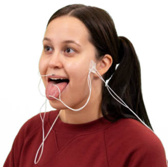
Figure 8: Example of electromagnetic articulography
