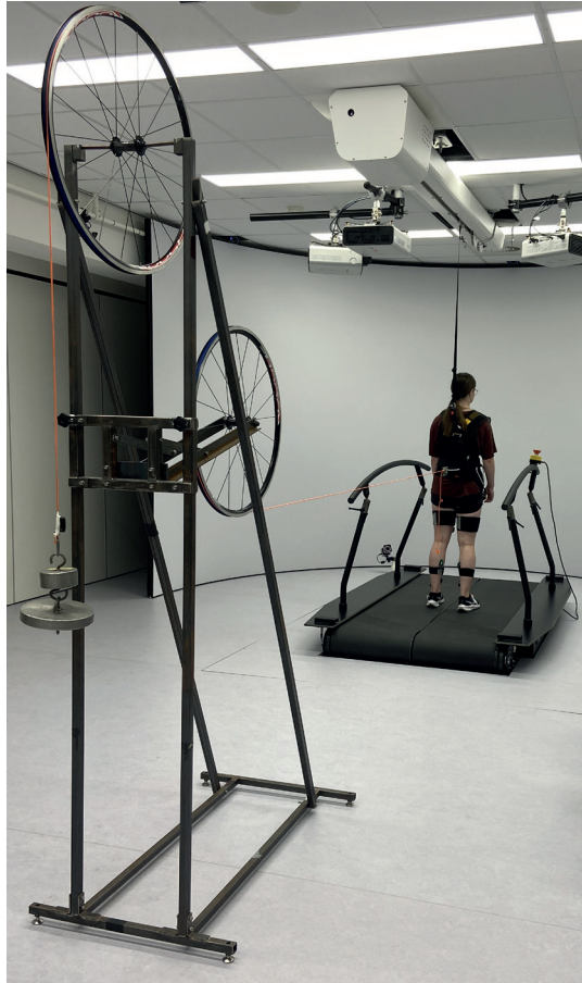
Fig 1: An illustration of the experimental set-up with the instrumented treadmill, safety harness system and the pulley system from 'right to left'.
