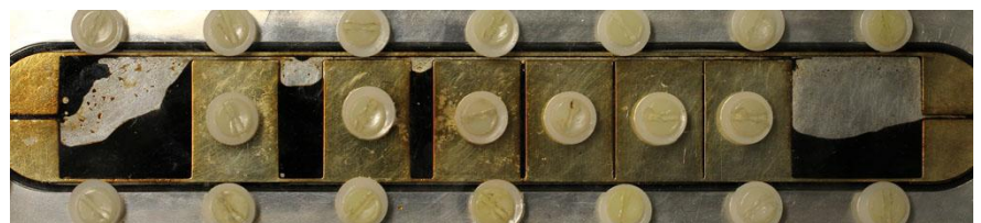
Figure 2. Flow-cell after 24h brine (30.000 ppm) flood, recovering 42% of oil in place
