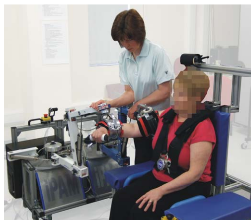
Fig. 1. The two iPAM robots are attached to a patient's arm
