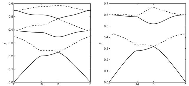
FIG. 1. Photonic band structure diagram of TM modes for a triangular lattice of air holes drilled in a dielectric medium ( $\epsilon = 13$ ,  $\mu = 1$ ). The holes have a diameter  $d = 0.80a$  (left) and  $d = 0.96a$  (right), where  $a$  denotes the lattice constant.
