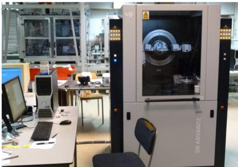
Fig. 3.4. D8 Advance X-ray diffractometer in Solid State Materials for Electronics group.
