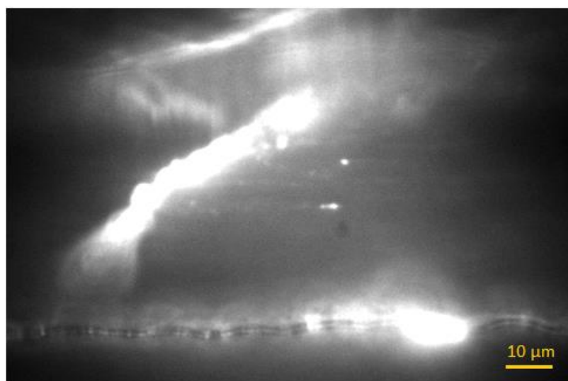
Figure 4.16: Fluorescence microscope image of a 'curtain' of multiple \lambda DNA molecules, stained with SYTOX Orange, hanging on a piece of 400 nm gold wire. Flow is coming in from the left at a flow rate of 1 \mu\text{l}/\text{min} . This image is a single frame, taken with an exposure time of 150 ms.
