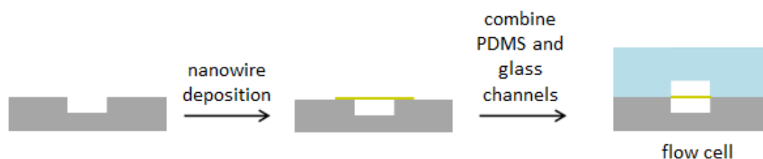
Figure 4.9: Illustration of flow cell device construction.
