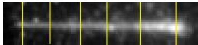
Figure 2.14: Average intensity sum over 2000 frames of a single \lambda DNA molecule at a flow rate of 10 \mu\text{l}/\text{min} , showing the cone-shaped figure of the DNA strand due to fluctuations because of flow. Yellow bars correspond to the data points in figure 2.15.
