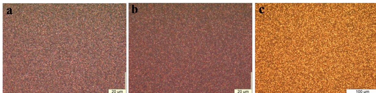
Figure 4.6. Optical micrographs of MAPbI 3 thin films deposited sequentially by dipping PbI 2 film that is blade coated under different conditions (of solution, substrate and annealing temperature) in MAI/IPA solution (10 mg/ml). The temperatures of the PbI 2 solution in DMF (1 M), substrate and annealing are respectively: a) 70, 50 and 70 °C b) 70, 80 and 70 °C (c) 100, 100 and 80 °C. The coating speed and duration of annealing are 5mm/s and 30 min respectively for each.
