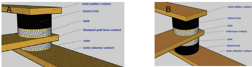
Figure 5 (A) Structure of the stamped base MIMIM. (B) Structure of the flip-over MIMIM. Compared to Figure 1 this structure uses two mutually connected large-area molecular junctions
