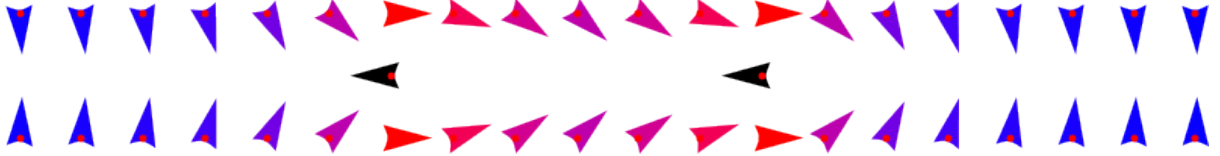
Figure 3.5: Let us now consider two layers (side view) with two Fe impurities in between (shown in black here). They both induce polarons in the above and below layers, where the spins are coloured proportional to their deviation from the vertical axis. The spins of the impurities are labeled by \mathbf{S}_1 and \mathbf{S}_2 , and we are interested in their effective interaction through the induced polarons.
