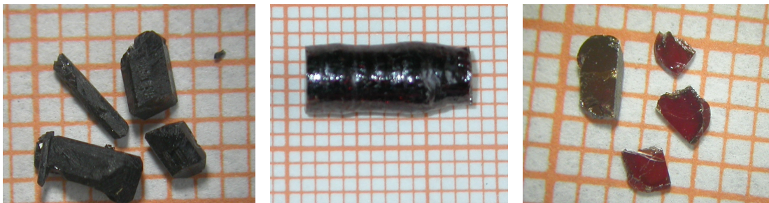
Figure 17: Flux grown crystals (left), and the floating zone crystals (middle and right).
