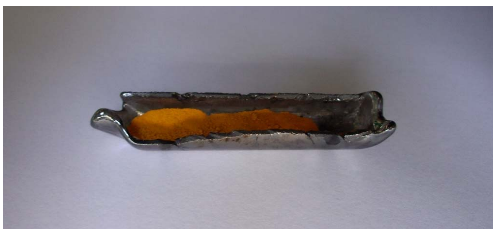
Figure 2-3: A photo of the quartz boat before being placed in the furnace. The reaction mixture ( V_2O_5+CrO_3 ) can be seen in the boat.
