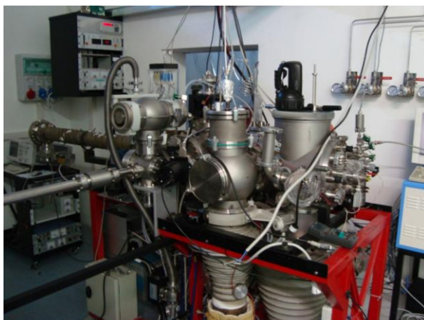
Figure 9: The SuMBD setup in Trento, Italy. The first chamber containing the source is located on the right side. The diffusion pumps are visible in the front and the elongated part at the back is the ToF.
