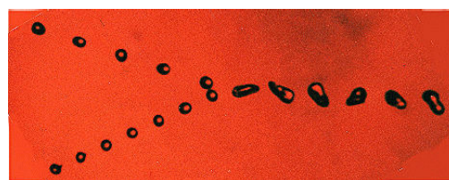
Fig. 2-5: Two streams of 120 \mu\text{m} water droplets merging into a single droplet stream at 20 kHz.
