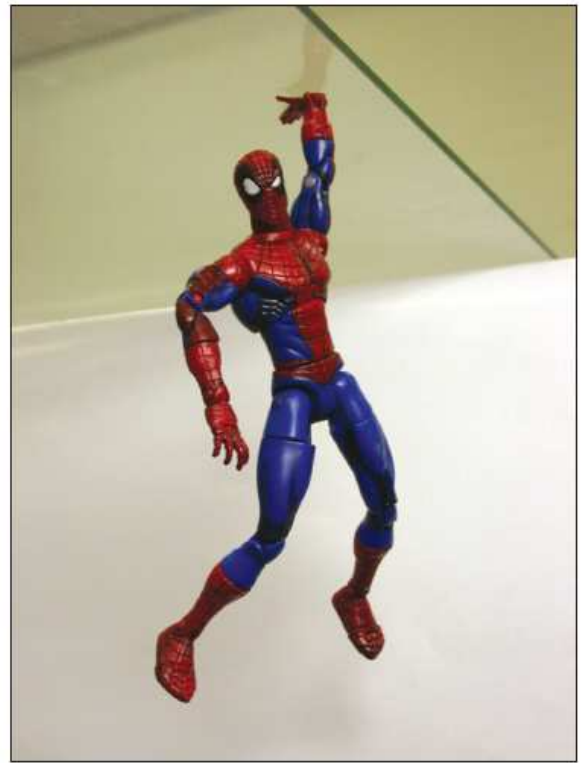
Figure 28. Re-attachable dry adhesives based on the gecko principle can find a variety of applications. The photo illustrates this point by showing a spider-man toy clinging with one of its hands to a horizontal glass plate. The toy (15 cm high; weighing 40 g) has its hand covered with the microfabricated gecko tape, which provides a \approx 0.5 \text{ cm}^2 contact with the glass and a carrying capacity of >100 \text{ g} . Note that the toy was already re-attached several times to various surfaces before this photo was taken [30].
