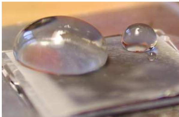
Figure 24. Superhydrophobic synthetic Geckopad specimen. Note the small water droplet on the right of the image which is almost circular. The large drop has a diameter of approximately 7\ \text{mm} [29].
