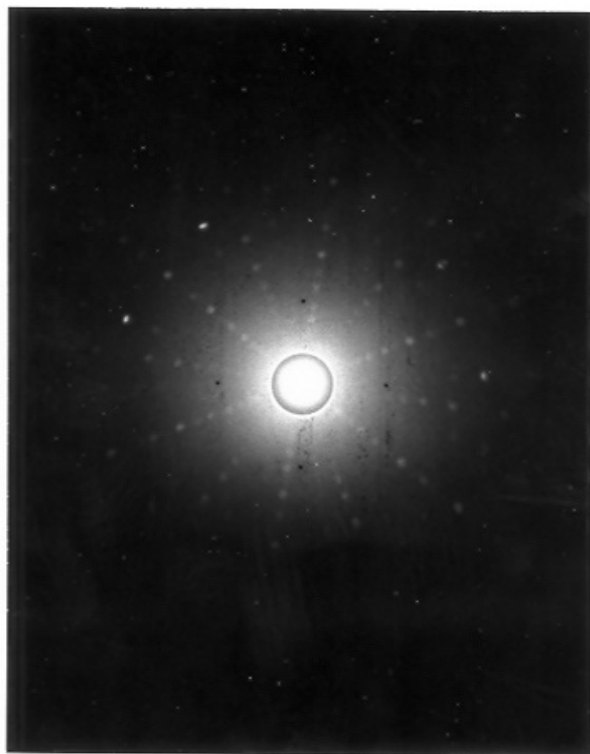
Fig. 24: X-ray Laue photograph of the Tb 2 Ti 2 O 7 -A crystal. The incoming beam is perpendicular to one of the natural faces of the crystal. The threefold rotation axis indicates that the natural facet is one of the \langle 111 \rangle planes of the crystal.
