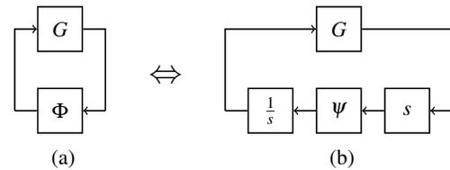
Figure 3: Feedback equivalence of a linear system with Preisach hysteresis in the feedback loop: (a). The original feedback loop as in (10); (b). The equivalent loop as in (14) which is based on the differential formulation as in (5).
