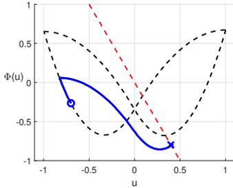
Figure 5: Input-output phase portrait of the closed-loop system from the numerical example. The dashed black line is the major hysteresis loop, the dashed red line is a linear line with the slope of  $\frac{1}{CA^{-1}B} = -2$ , and the solid blue line is the simulation data with initial values  $(u(0), y(0))$  marked by a circle and final values  $(u(\infty), y(\infty))$  marked by a cross.
