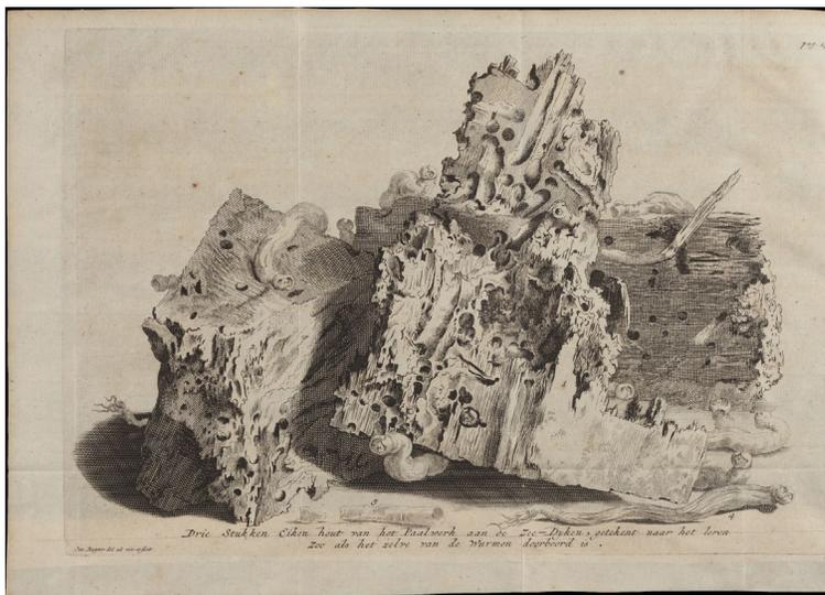
FIGURE 2 Fold-out in *Europische Mercurius* 43/1 (1732), between pp. 296-297, representing oak tree poles affected by shipworm. Copy University of Groningen Library (photograph Dirk Fennema, Haren, Netherlands).
