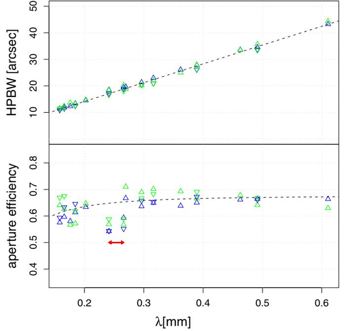
**Fig. 3.** HPBW and aperture efficiencies observed as a function of wavelength towards the planet Mars. Blue and green symbols represent observed values for horizontal and vertical polarization, respectively, whereas up and down pointing triangles distinguish two different observing runs. The black dashed lines represent fits to the relations described by Eqs. (3) and (1), resp. Observations in band 5 (marked with the red arrow) were excluded from the fit to the aperture efficiencies.
