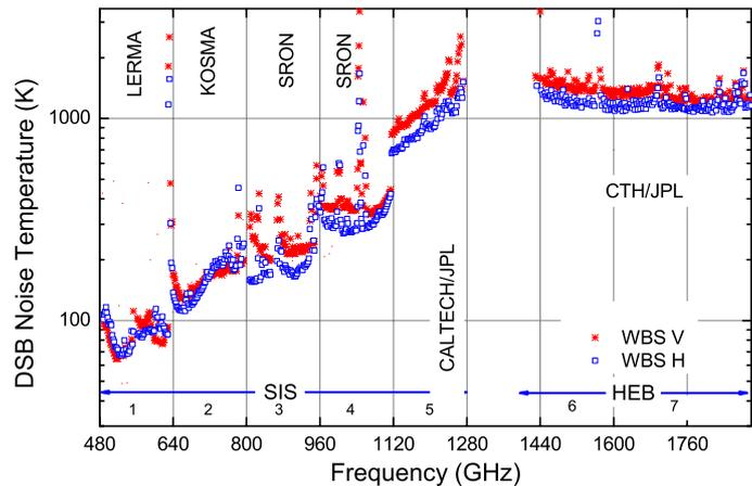
**Fig. 2.** System temperature of HIFI for H-polarization (blue squares) and V-polarization (red circles). The vertical bars indicate the frequency boundaries of the different mixer bands. Also indicated are the institutes responsible for the design and implementation of the different mixers.
