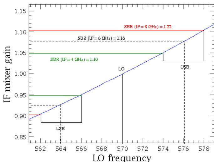
**Fig. A.1.** Deviations in sideband ratio with large sideband separation.
