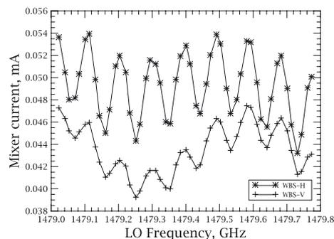
**Fig. 5.** Plot of the mixer currents for both H and V mixers. For this test the LO power is kept constant and the LO frequency is changed. In this plot two standing waves are apparent; a 92 MHz modulation corresponding to a distance between the LO source unit and the mixer focus and a 680 MHz period standing wave corresponding to a reflection between the diplexer rooftop mirror and the mixer focus.
