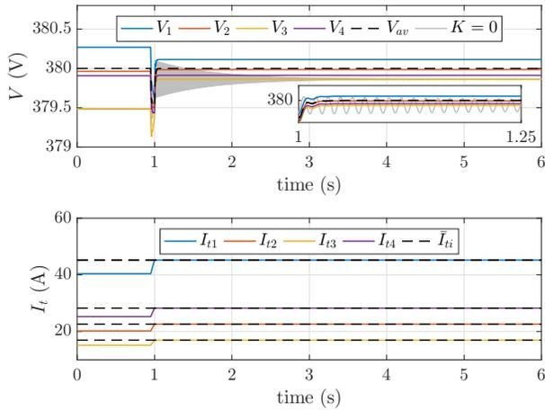
Fig. 3. (Proposed controller) From the top: voltage at the PCC of each DGU together with the weighted average value (dashed line) and the voltage at the PCC of DGU 3 when  $K = \mathbf{0}$  (grey line); generated currents together with the corresponding values (dashed lines) that correspond to (proportional) current sharing for  $t > 1$ .
