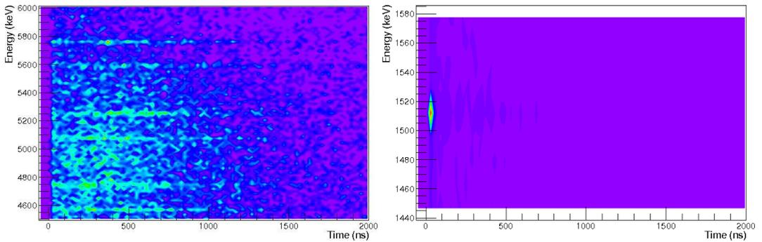
**Figure 4.** Observed X-ray transitions as a function of time after the muon entered the cell. Left:  $^{197}\text{Au}$  2p-1s muonic X-rays at 5764.9 keV and 5595.0 keV. The single and double escape peaks are also visible at lower energies. Right:  $^{63}\text{Cu}$  2p-1s muonic X-rays at 1508.05 keV and 1514.45 keV.
