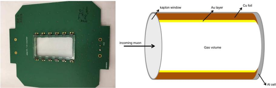
**Figure 2.** Left: Picture of the BC-400 plastic scintillator used to trigger the entrance of the muons in the cell volume. The twelve silicon photomultipliers used for the readout are visible. Right: Schematic view of the gas cell.
