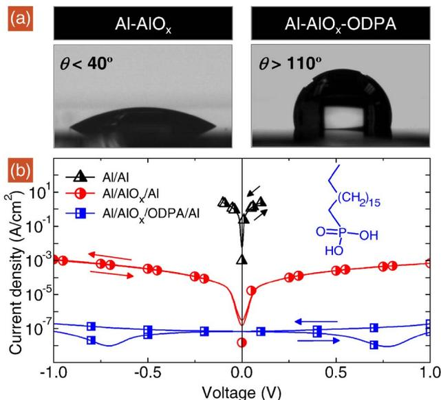
FIG. 1. (Color online) (a) Water droplets on Al-AIO<sub>x</sub> (left) and Al-AIO<sub>x</sub>-ODPA (right). (b) Current density vs bias voltage for diodes fabricated with untreated Al electrodes (triangles), oxidized bottom electrode (circles) and ODPA functionalised Al-AIO<sub>x</sub> bottom electrode (squares). Inset: molecular structure of ODPA.
