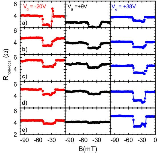
FIG. 3 (color online). The drift effect in a graphene spin valve. The gate voltage  $V_g$  varies from left to right and it is indicated for each column. The dc electric current varies from top to down as: (a)  $I_{dc} = -40 \mu\text{A}$ , (b)  $-20 \mu\text{A}$ , (c)  $0 \mu\text{A}$ , (d)  $+20 \mu\text{A}$ , (e)  $+40 \mu\text{A}$ . For clarity only the negative side of the spin valve measurements are plotted.
