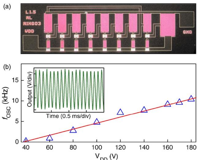
FIG. 4. (Color online) (a) Micrograph of the seven-stage ring oscillator based on type II transistors employing  $L=1.5\ \mu\text{m}$  as the design rule. (b) Oscillation frequency vs  $V_{\text{DD}}$  for a seven-stage ring oscillator based on 1. Inset: output signal at  $V_{\text{DD}}=170\ \text{V}$ .
