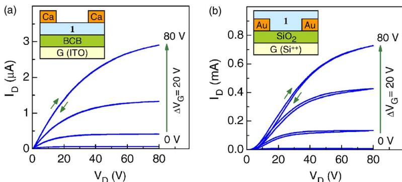
FIG. 3. (Color online) Output characteristics for a type I (a) and a type II (b) transistors based on 1. The channel dimensions for the type I device are  $L=60$   $\mu\text{m}$  and  $W=1$  mm. For the type II transistor  $L=10$   $\mu\text{m}$ ,  $W=20$  mm. Insets: schematic structures of type I (a) and type II (b) transistors tested.
