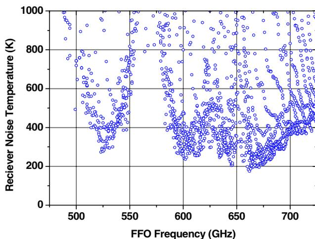
**Figure 2.** Uncorrected DSB noise temperature of the SIR as a function of FFO frequency measured at different FFO bias currents that results in various SIS pumping levels ( $T_{\text{BATH}} = 2.1$  K,  $V_{\text{SIS}} = 2.2$  mV, IF = 4.3 GHz).
