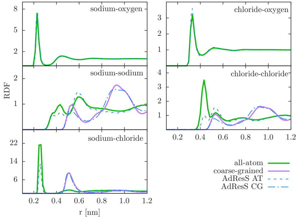
**Fig. 3.** Radial distribution functions (RDFs) of sodium-oxygen, chloride-oxygen, sodium-sodium, chloride-chloride, and sodium-chloride for the bulk solvent system. The AdResS RDFs match well the reference all-atom and coarse-grained simulation results. Labels “AdResS AT” and “AdResS CG” denote the AdResS domain, i.e. the atomistic and coarse-grained regions, respectively.
