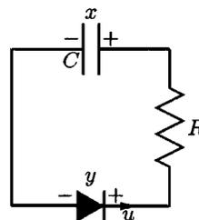
Fig. 3. A circuit containing a negative resistor.
