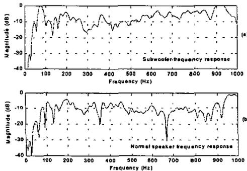
Fig. 2. Estimated secondary path frequency response. (a) Secondary path employing sub-woofer; (b) Secondary path employing standard speaker
