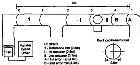
Fig. 1. Experimental duct configuration
