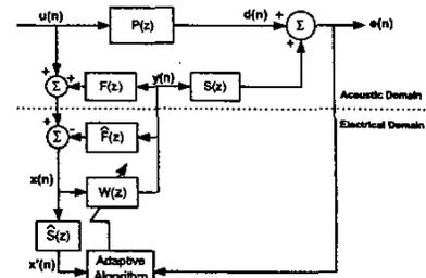
Fig. 3. Filtered-x approach block diagram for ANC with feedback neutralization filter.
