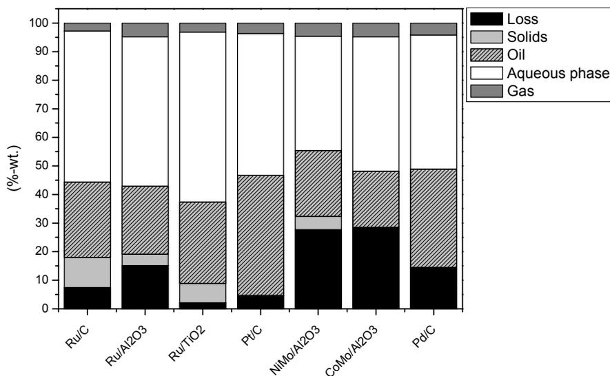
Figure 2. Mass balances for the mild HDO of pyrolysis oil with different catalysts (250 °C, 100 bar, 4 h).
