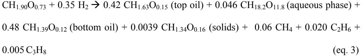
On basis of these data the hydrogen uptake was estimated at 400 NL/kg dry pyrolysis oil for Ru/C. As expected on the basis of the elemental composition of the oil phases and the composition of the gas phase (more CH<sub>4</sub>), the uptake for Pd/C was noticeably higher and about 450 NL H<sub>2</sub>/kg dry pyrolysis oil.
