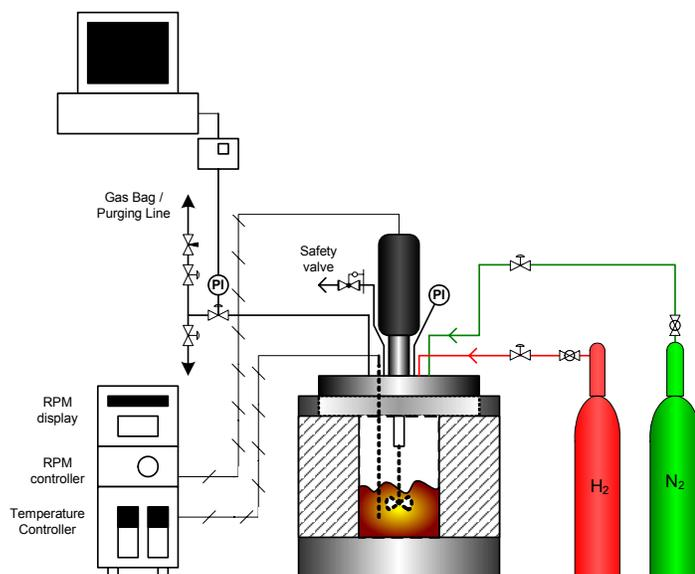
Figure 1. Schematic representation of the autoclave setup.
