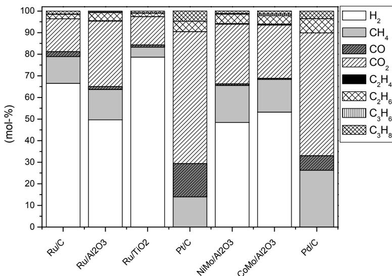
Figure 7. Gas composition for the deep HDO of pyrolysis (350 °C, 200 bar, 4h) using various catalysts.
