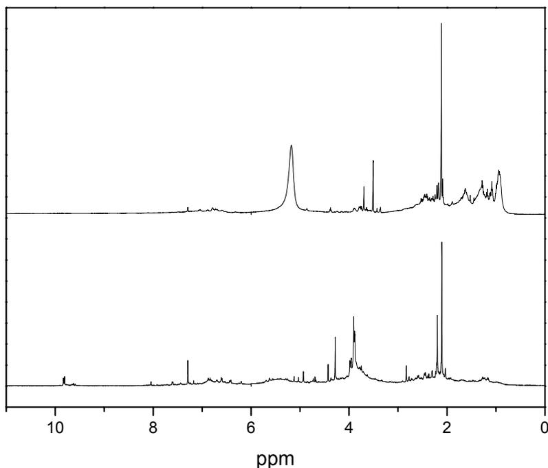
Figure 10. <sup>1</sup>H-NMR analysis of pyrolysis oil (bottom) and HDO oil (top, Ru/C, 350 °C, 200 bar, 4 h) in CDCl<sub>3</sub>.
