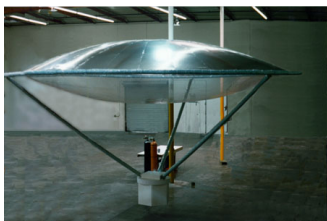
Fig. 1. An inflatable space reflector test setup of the company L'garde ( www.lgarde.com )
