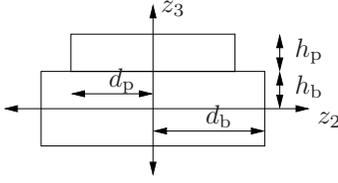
Fig. 1. Cross sectional area of the composite
