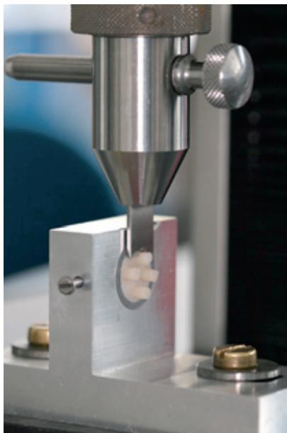
**Fig 2** Representative specimen mounted in the jig of the universal testing machine with adhesive interface submitted to shear force.
