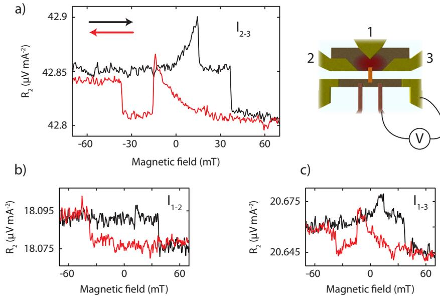
Figure 5.3: **Measured voltage from the Py-NiCr thermocouple by selectively switching the magnetizations by an antiparallel magnetic field in a lateral spin valve.** The right thermocouple is measured when the Joule heating current is sent **a)** parallel to the magnetization  $M_1$ , **b)** under a 45 degree angle and **c)** under a -45 degree angle. The results were calculated by sending an r.m.s charge current of 1.5 mA. The other thermocouple was also measured and shows similar results.
