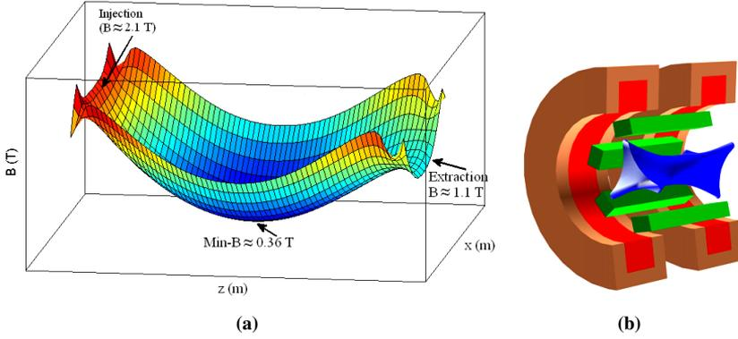
**Figure 3.2:** Typical (*Min-B*) magnetic structure of a 14.1 GHz ECR ion source (a) and 3D view of ECR ion source magnetic field configuration (figure taken from Ref. [64]) (b).
