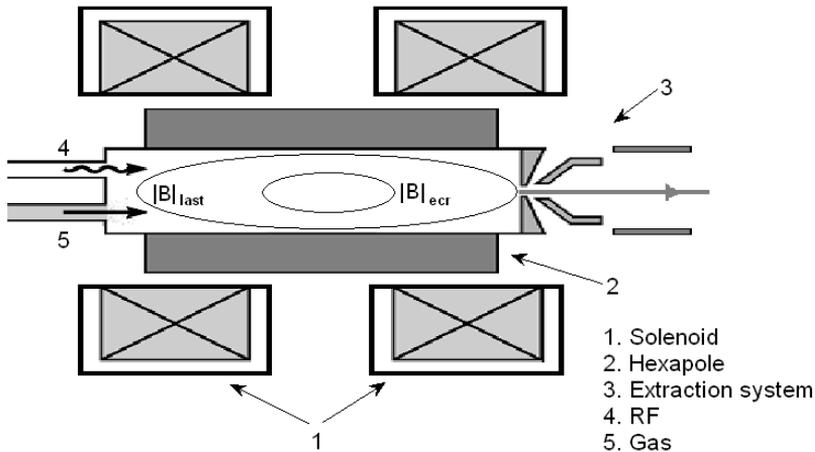
Figure 3.1: Schematic view of an ECR Ion Source.
