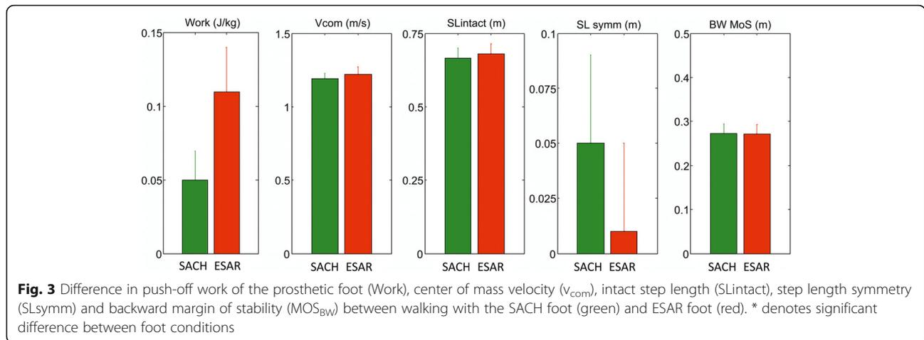
step length improved step length symmetry ( $p < 0.001$ ). The difference in step length between the intact and prosthetic step, reduced from  $0.05 \pm 0.04$  m while walking with the SACH foot, to only  $0.01 \pm 0.04$  m while walking with the ESAR foot.
