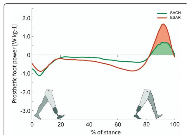
**Fig. 2** Push-off power of the prosthetic foot as a function of normalized stance time. The ESAR foot (red) generates negative power, storing elastic energy, in midstance and generates a higher positive push-off power, returning, more elastic energy during push-off compared to the SACH foot (green). The coloured surface below the power profile indicates the amount of work delivered during push-off (Figure amended from Wezenberg et al. 2014 [9])
