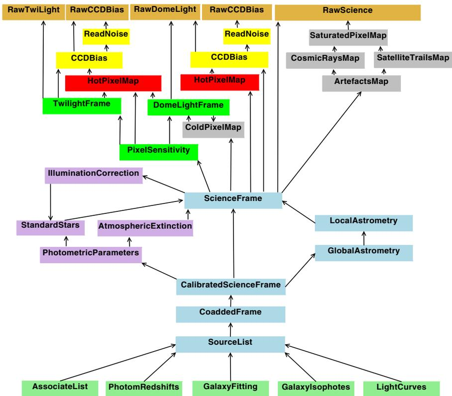
**Fig. 3** Overview of classes of data objects. Data objects not only contain the survey products denoted by familiar names in wide-field imaging. They also carry the information how they, as requested target, can be created out of other survey objects, illustrated by the *arrows*. Underlying is an object model that captures the relationship between requested information and the physics of the atmosphere-to-detector observational system
