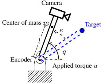
Fig. 1: Illustrative example of output regulation problem of single-link manipulator using error and velocity feedback.
