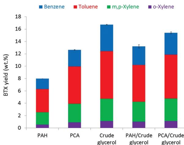
**Fig. 3** Average BTX yields (wt% relative to feed intake) obtained after *ex situ* catalytic pyrolysis of crude glycerol and co-pyrolysis with PAH or PCA (1:1 wt ratio, total weight of 1 g) in the presence of the H-ZSM-5 catalyst (1:3 feed mix: catalyst wt ratio, 550 °C). Error bars indicate standard deviation.
