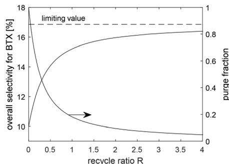
Fig. 6 Overall selectivity percentage of BTX and its limiting value vs. the recycle ratio (left axis), and fractional purge vs. the recycle ratio (right axis).
