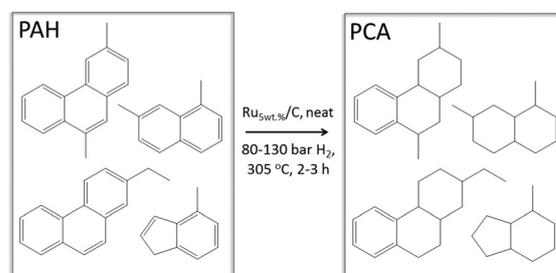
**Fig. 2** Chemistry for the catalytic hydrogenation of the isolated PAH fraction, showing representative components as well as the reduced fraction (collectively denoted as polycyclic aliphatics or PCAs).
