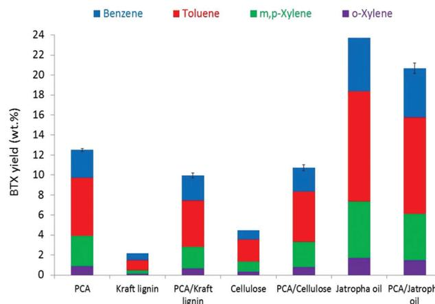
**Fig. 4** Average BTX (wt% relative to feed intake) obtained after *ex situ* catalytic pyrolysis of Kraft lignin, cellulose and Jatropha oil, and co-pyrolysis of each biomass feedstock with PCA (1:1 wt ratio, total weight of 1 g) in the presence of the H-ZSM-5 catalyst (1:3 biomass mix: catalyst wt ratio, 550 °C). Error bars indicate standard deviation.
