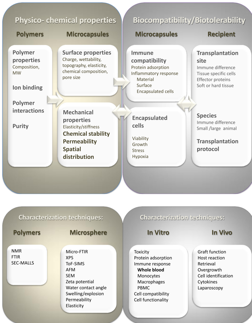
Fig. 1. Determinants of the “optimal window” for functional characterization of microspheres for cell encapsulation. Upper panel: physico-chemical properties and relation to biocompatibility/biotolerability. Lower panel: characterization methods/properties for polymers and microspheres related to physico-chemical characteristics, in vitro immune and in vivo specific properties related to biocompatibility/biotolerability. Arrows point at the principal mutual dependency of determinants. The abbreviations are explained in the text.
