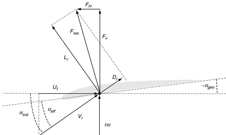
**Figure 5:** Forces and velocities on a blade-element:  $\alpha_{eff}$  = effective angle of attack;  $\alpha_{geo}$  = geometric angle of attack;  $\alpha_{ind}$  = induced angle of attack;  $U_f$  = free flow velocity;  $v_r$  = effective velocity;  $r$  = radial distance of wing element;  $\omega$  = angular velocity of the wing;  $L_r$  = lift;  $D_r$  = drag;  $F_{res}$  = resulting force;  $F_H$  = horizontal force component;  $F_V$  = vertical force component.
