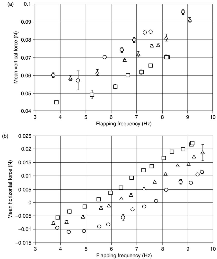
**Figure 6:** Mean forces of the flapping wings for different  $U_f$  ( $n = 3$ ; squares = 2.28 m/s ; triangles = 2.57 m/s ; circles = 2.84 m/s). (a) Mean vertical force ( $\bar{F}_V$ ) increases with flapping frequency. (b) Mean horizontal force ( $\bar{F}_H$ ) increases with flapping frequency and becomes positive for high flapping frequencies. Here, the MAV creates "net thrust"
