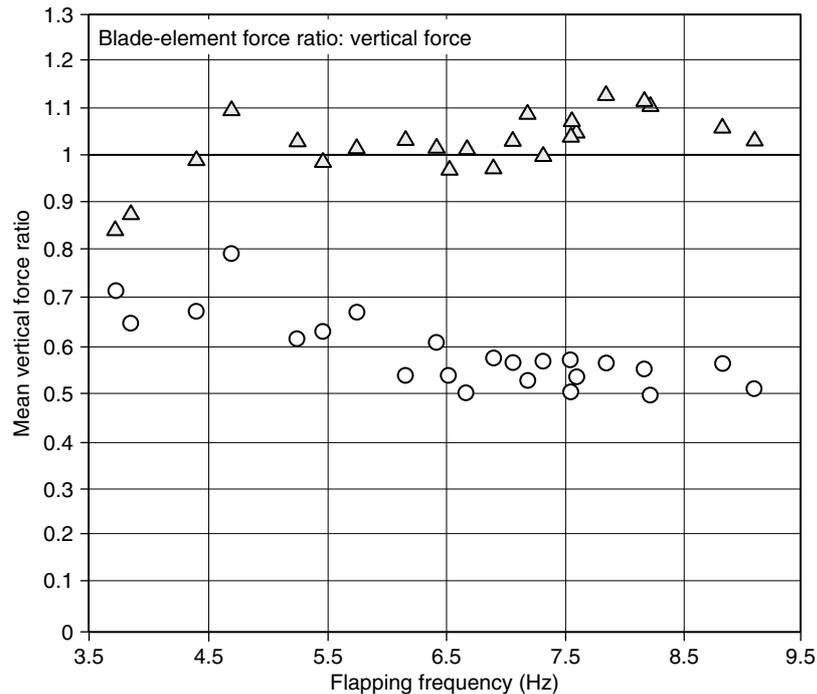
**Figure 9:** Force ratio:  $\overline{F}_V$  (blade-element analysis) divided by  $\overline{F}_V$  (experiment). Data for different free flow velocities was pooled. Circles: "Steady" coefficients underestimate  $\overline{F}_V$  by a factor of up to two. Triangles: "Vortex-lift" coefficients deviate by maximally 13% (excluding measurements at frequencies close to the resonant frequency of the balance system), and on average by  $2.9\% \pm 6.9\%$  ( $n = 23$ ).
