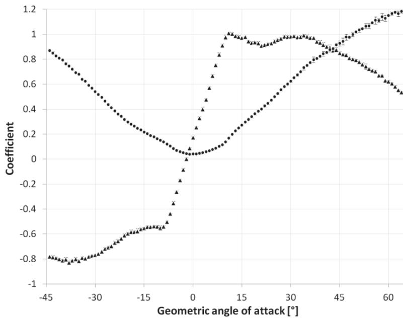
**Figure 3:** “Steady coefficients”. Lift (triangles) and drag (circles) coefficient of the wings in steady-flow for geometric angles of attack between  $-45^\circ$  and  $65^\circ$  ( $Re = 1.4 \cdot 10^4$ , step size =  $1^\circ$ ,  $n = 3$ ).
