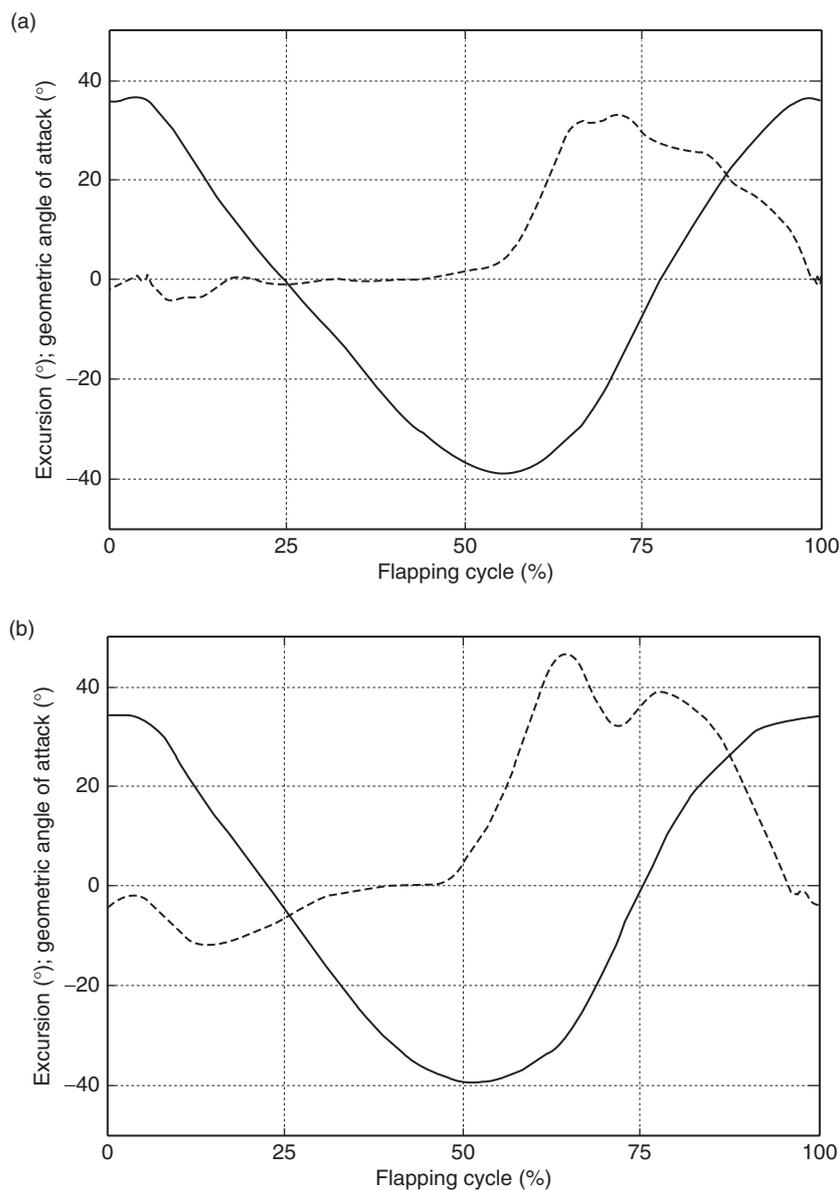
**Figure 2:** Wing excursion (solid line) and geometric angle of attack (angle between  $U_f$  and wing chord; dashed line). (a) Wing kinematics for a flapping frequency of 3.65 Hz in 2.28 m/s flow. (b) Wing kinematics for a flapping frequency of 7.61 Hz in 2.84 m/s flow. The kinematics change at increasing flapping frequency and free flow velocity due to increasing aerodynamic and inertial load and some elasticity in the mechanical design.
