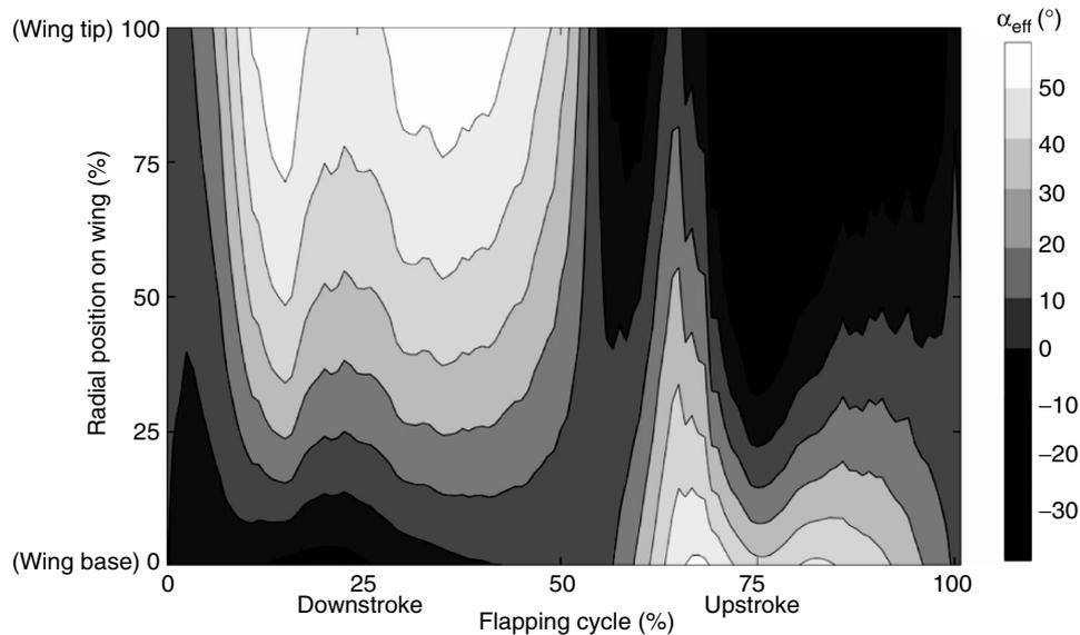
**Figure 12:** Effective angle of attack as a function of span wise position and flapping cycle. During downstroke and close to the wing tip, the effective angle of attack reaches  $50^\circ$  (see greyscale bar at the right)
