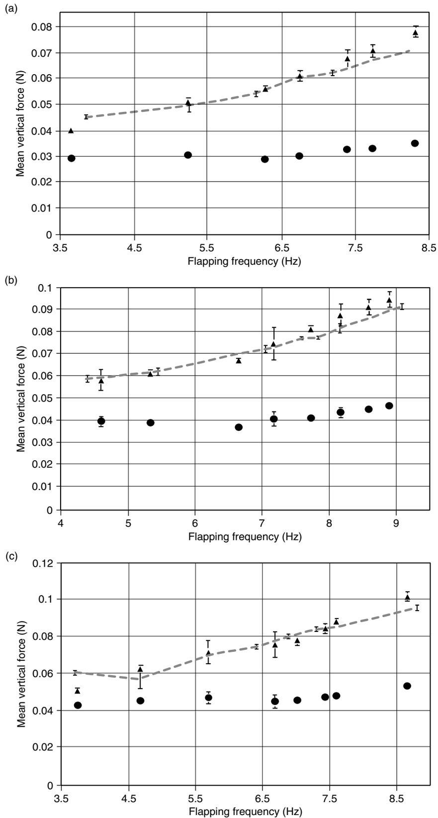
**Figure 8:** Results of  $\overline{F}_V$  for of the blade-element analysis with “steady” (circles) and “vortex-lift” (triangles) force coefficients compared to force balance measurements (dashed line). (a)  $U_f = 2.28$  m/s, (b)  $U_f = 2.57$  m/s, (c)  $U_f = 2.84$  m/s. In all cases, “steady” coefficients underestimate mean vertical force, whereas “vortex-lift” coefficients show a good agreement.
