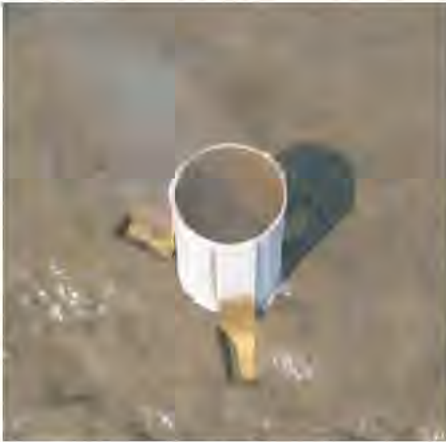
Figure 15. A 'cryolander' has been designed to sample the sediment without disturbing the surface layer. The sediment is rapidly frozen by the addition of liquid nitrogen. In the laboratory, the top layer is sliced in small coupes of \sim 100 \mu\text{m} , which thereupon can be analysed for their pigment content.
