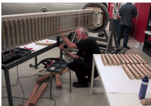
Figure 14. Repairing the 2.5 MV high-voltage generator.
