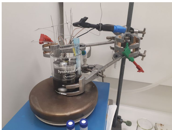
Figure 5: Top panel: Home-made electrochemical cell with a stack of four paired porous graphite electrodes for gram-scale synthesis.
