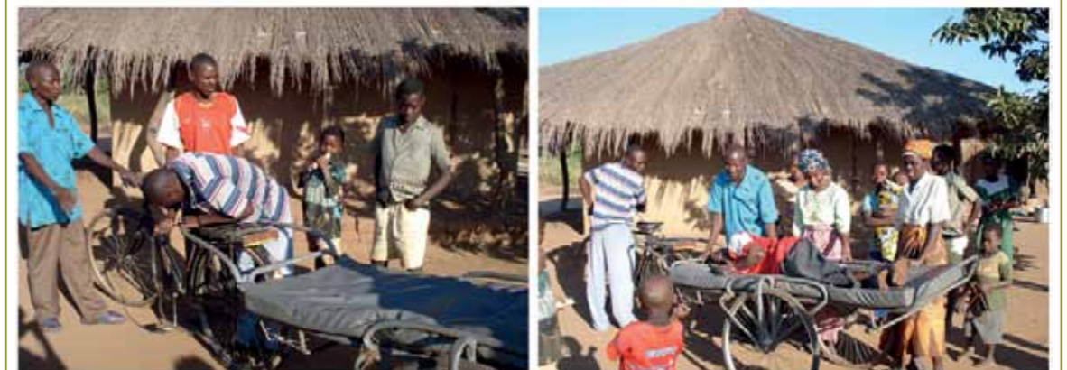
Figure 6: An Adapted Bicycle Ambulance Photograph: Mary Sibande
