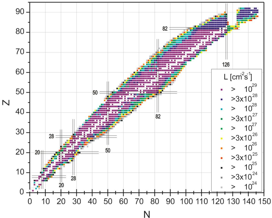
**Figure EX.1:** Luminosities expected at the FAIR NESR storage ring using an internal hydrogen gas-jet target of  $10^{14}$  atoms/cm<sup>2</sup>.
