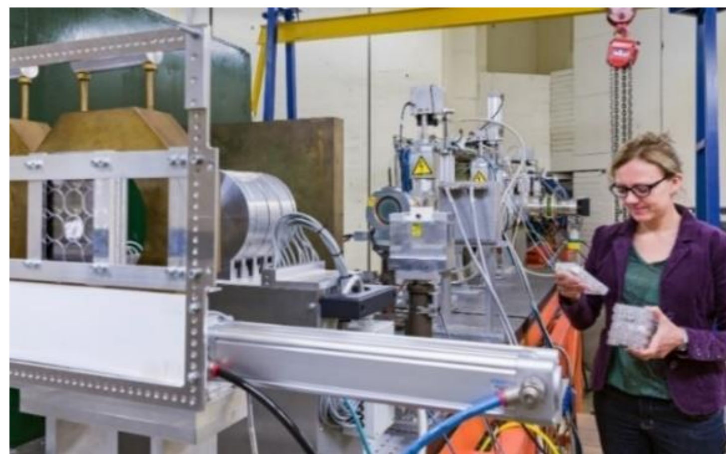
In-air heavy ion irradiation facility for radiation hardness testing & radiobiological research
