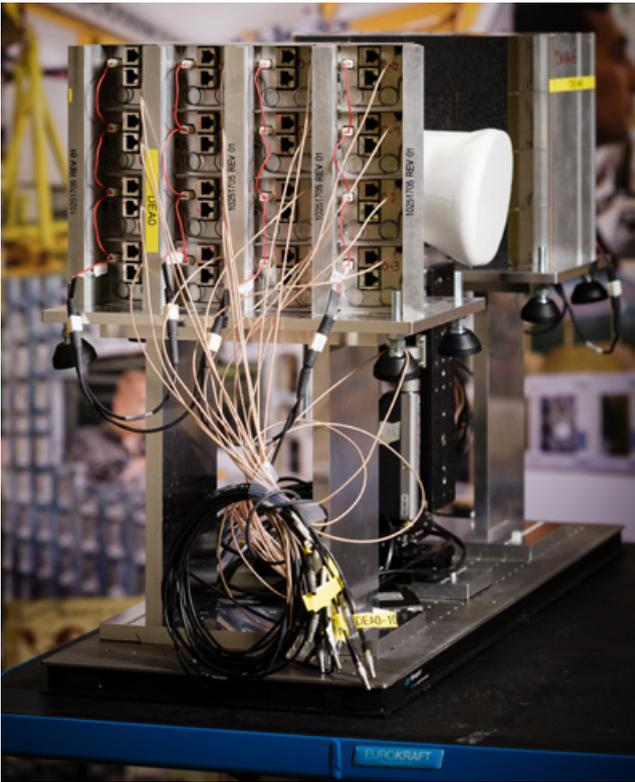
The test set-up used by Peter Dendooven and Ikechi Ozoemelum in the laboratory: two PET ring elements surround a (polystyrene) model of a human head.
