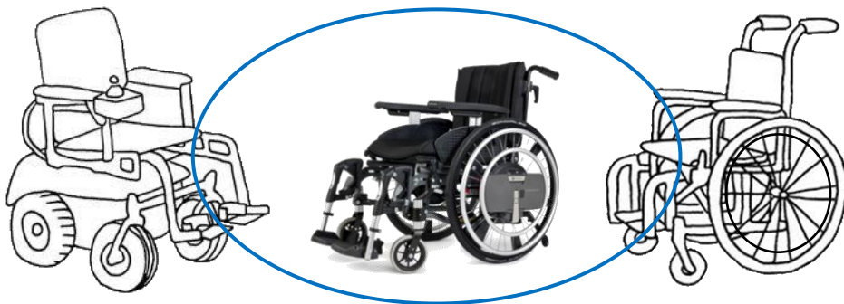
Figure 1 - The power-assisted wheelchair ( Mid ) is an intermediate between the powered ( Left ) and hand-rim wheelchair ( Right ).
