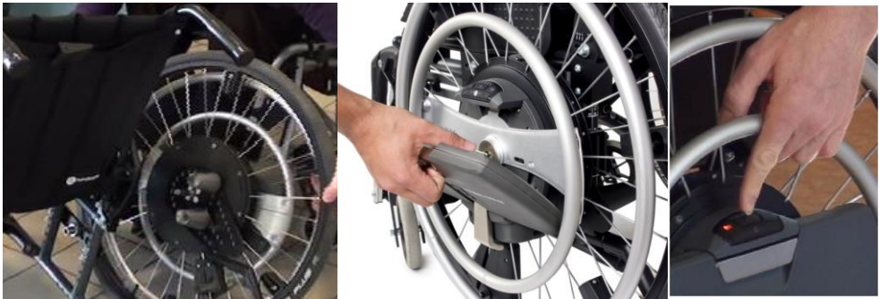
Figure 2 - Left - Mounting mechanism for attachment to varying wheelchair frames. Mid - Motor and removable battery pack positioned around the axis. Right - Upper rim for power-assisted propulsion, lower rim for completely powered propulsion. For both rims the amount of additional power can be switched between 3 modes.
