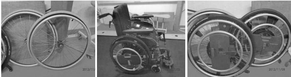
Figure 1 - Left Manual wheels; Mid - power-assisted wheels with conventional motor, mounted on the wheelchair frame; Right - power-assisted wheels with extra-power motor attached.
