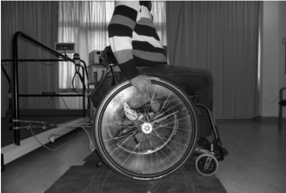
Figure 3. Set-up of the isometric wheelchair push used to assess isometric strength. See chapter 5 for a schematic presentation of the set-up.
