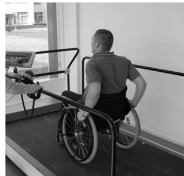
Figure 3. Wheelchair propulsion using a motor-driven treadmill.
