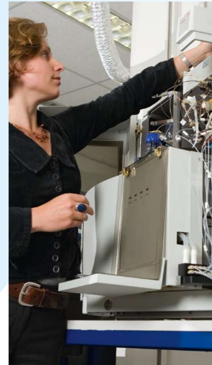
Separation and analysis of tiny amounts of molecules by nano-flow liquid chromatography and mass spectrometry.
